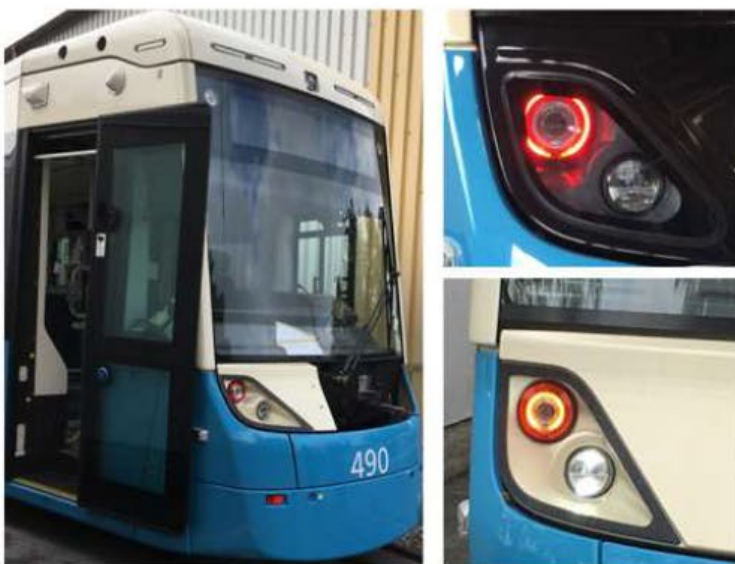
Photo: shows area with covered lights, below them the 3D printed modified solution
