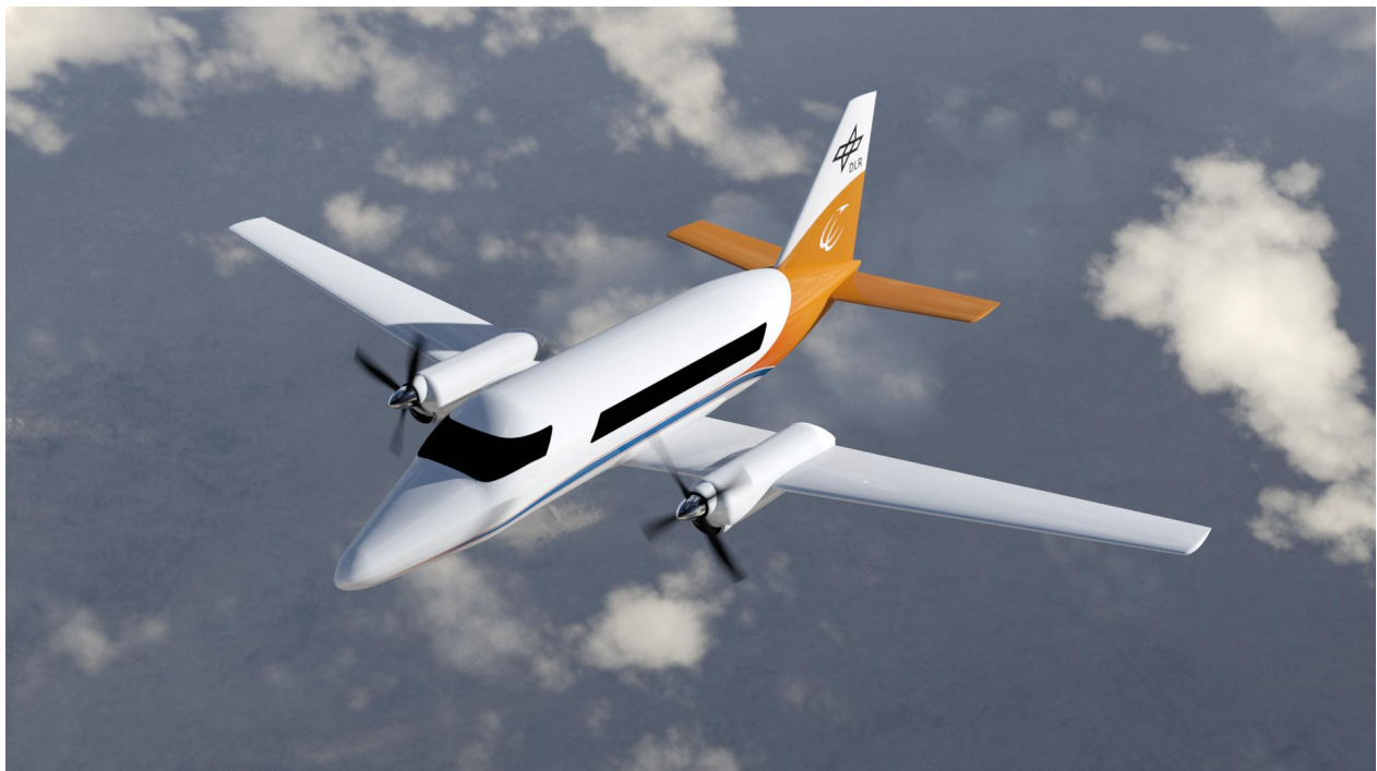
Conceptual study of a hybrid electric 19-seater aircraft as part of the CoCoRe research project. (Credit: DLR/BHL)
