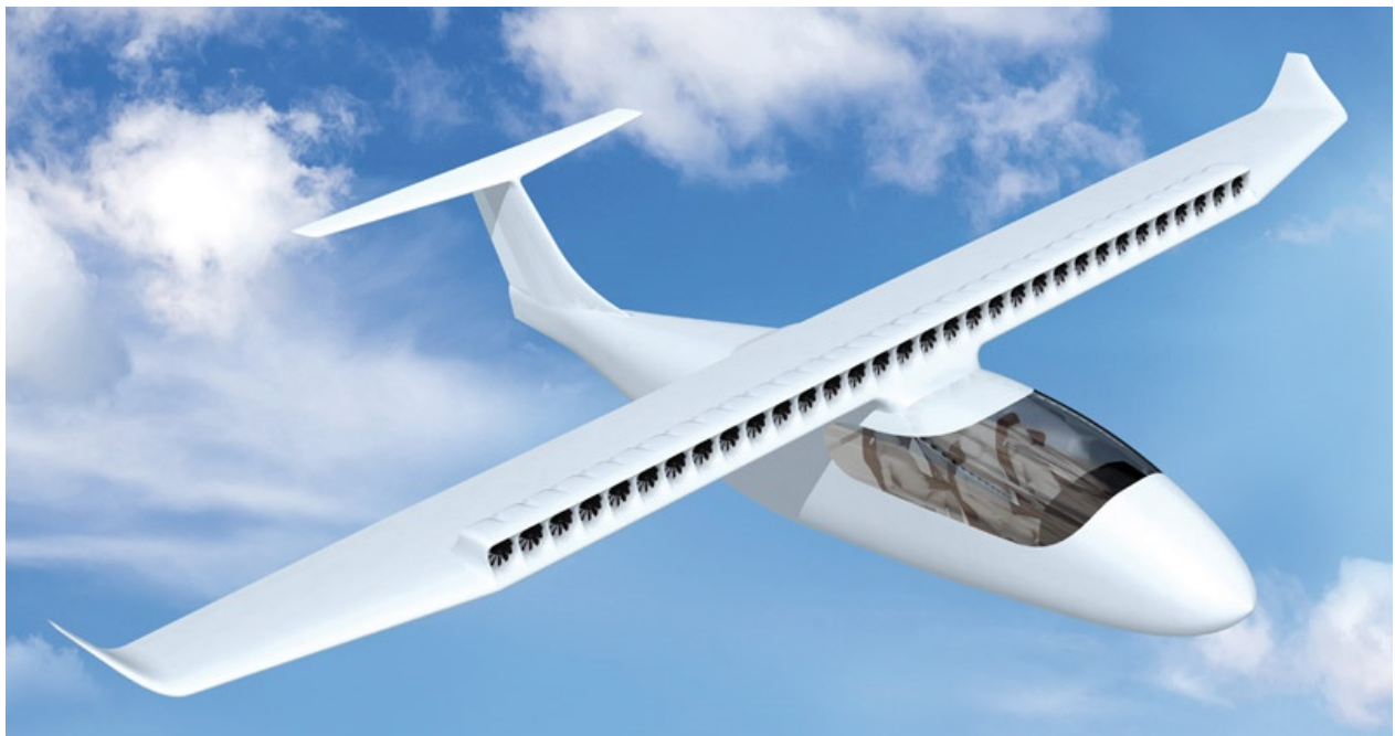
A concept of distributed electric propulsion on a regional aircraft demonstrator designed for transporting between 4 and 6 people over 500 km in 2 hours. (Credit: Onera)
