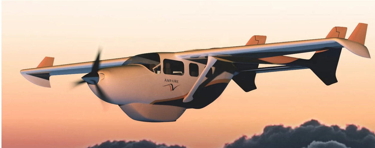
The Electric EEL, a modified Cessna 337. (Credit: Ampaire)
