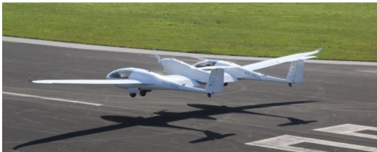
The German research institute DLR has equipped this flying test platform with a 45-kW hydrogen fuel cell combined with a 22-kWh battery. The aircraft can cruise at 145 km/h and has a range of 750 – 1 500 km. (Credit: DLR)
