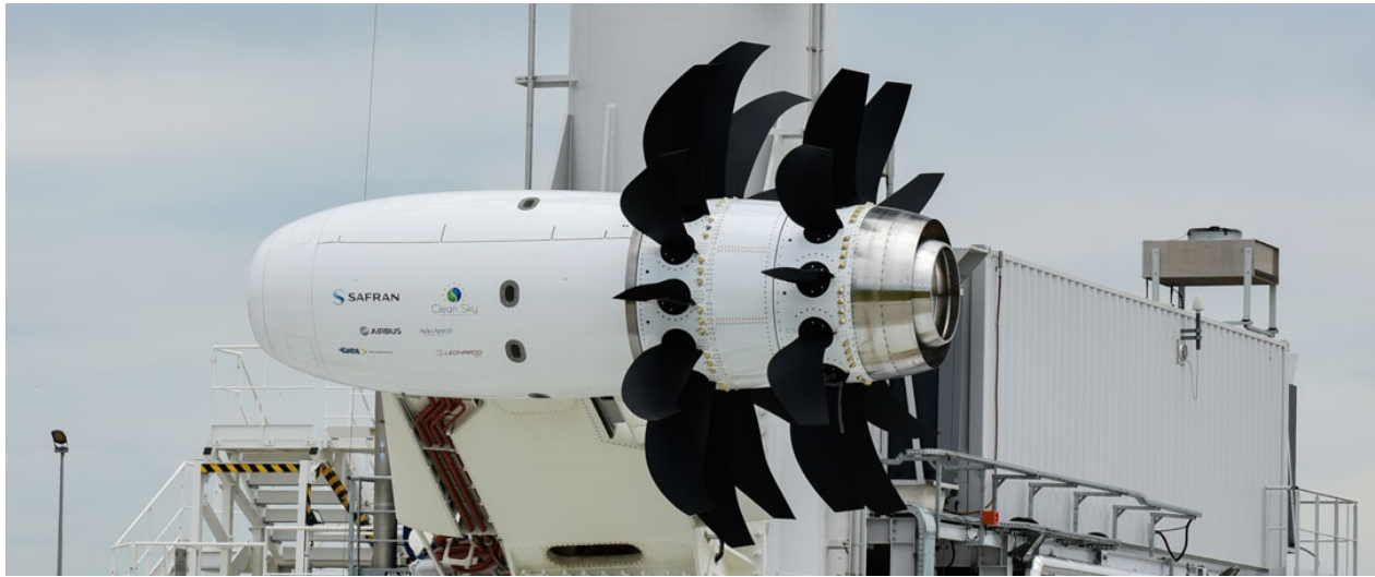
Safran open-rotor demonstrator. The engine configuration could burn 15 percent less fuel than the CFM Leap. (Credit: Safran)
