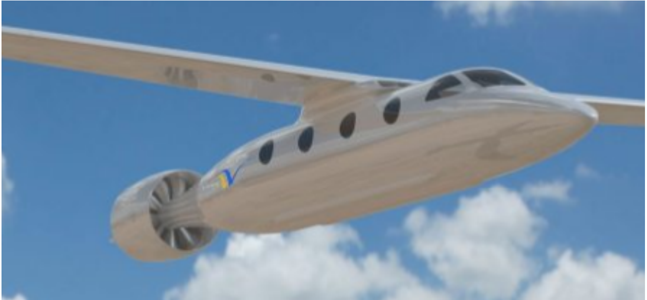
The Ampaire team has designed their futuristic aircraft with a tail electric ducted fan. (Credit: Ampaire)
