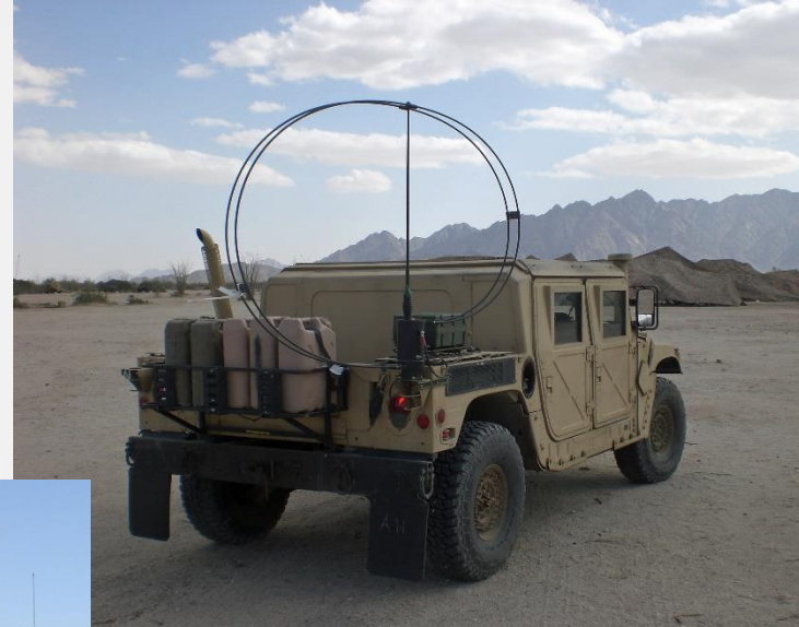
HF230L-OTM HF Loop Antenna. Below HIMARS
