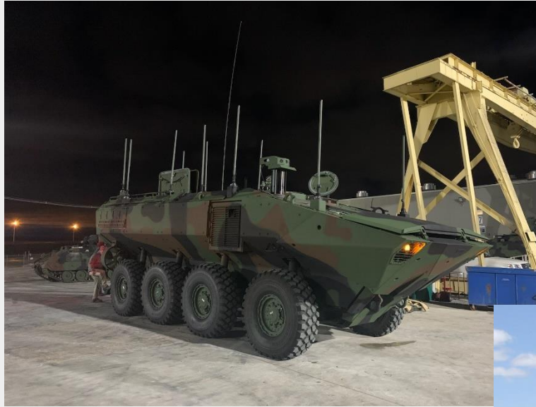
VHF302600TB Antennas on US Marines Amphibious Combat Vehicle (ACV)
