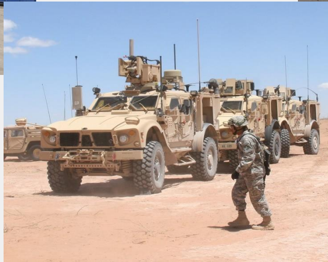
VHF30512CEF Antennas on MRAP
